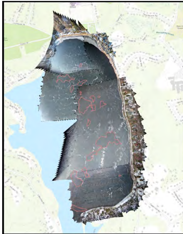
LMAC Figure BG-11: Lake Massapoag Ice Holes from Pilot Drone Survey and Airplane
