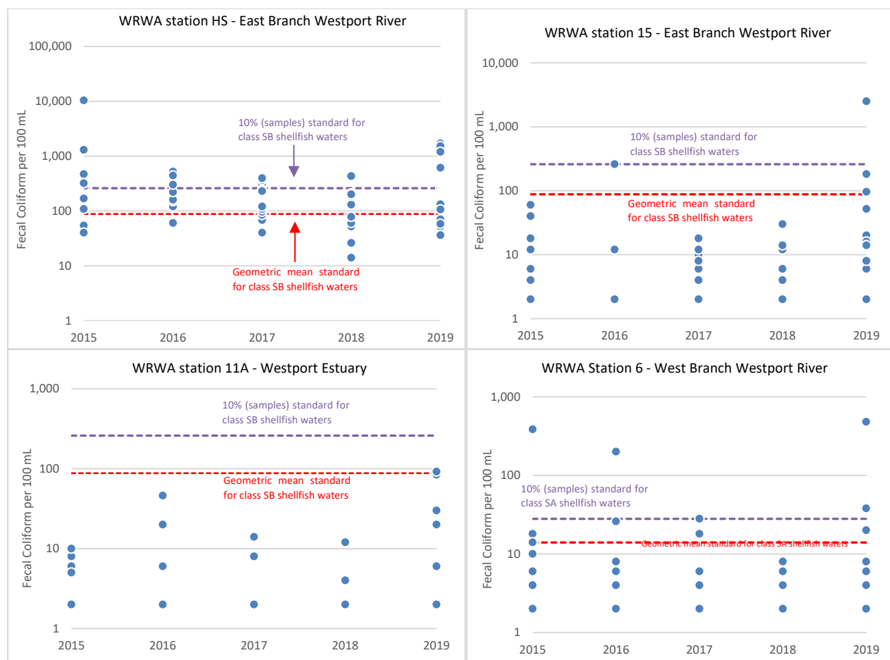
Figure A-6: Westport River Watershed Alliance FC monitoring data (summer 2015–2019) and associated shellfish waters criteria (classes SA and SB) for selected monitoring stations in Westport River watershed (Adapted from NRCS, 2021)
